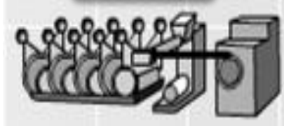
Topping of bead wire; extrusion of bead filler
